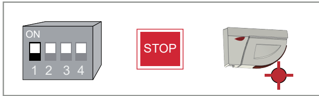
RELAY 1: STOP-impuls on the opening side of the door
